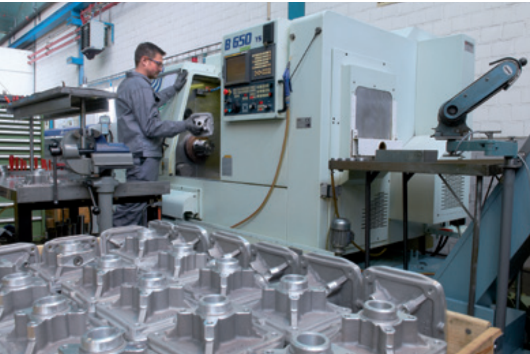
Production of cylinder parts on dual spindle turning center
